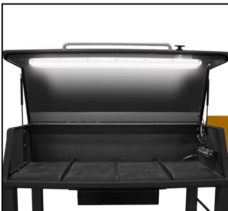
Built-in work light to facilitate to see the hose being tested.
